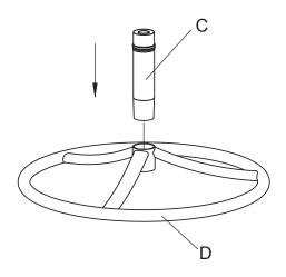
• Push the center post (C) down firmly and twist it left and right as necessary.
