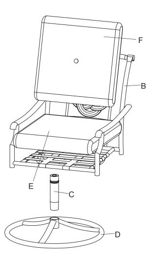
**1** Inserting the center post into the swivel base
