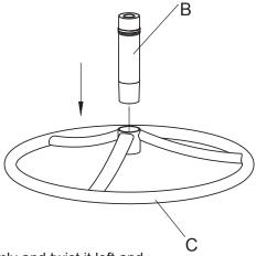
• Push the center post (B) down firmly and twist it left and right as necessary.
