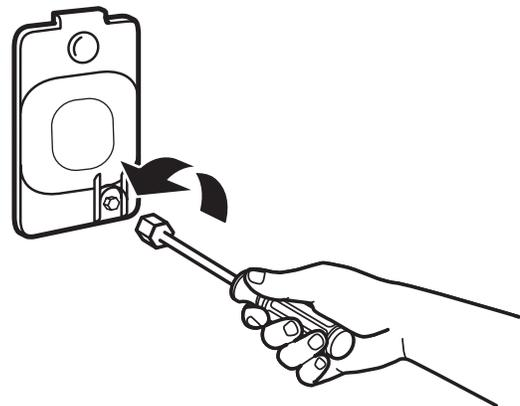
3. Turn bulb counterclockwise. Replace the bulb with a 10-watt appliance bulb only. Replace the cover and secure with the screw.
