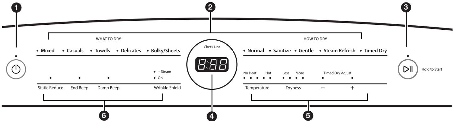
**NOTE:** The control panel features a sensitive surface that responds to a light touch of your finger. To ensure your selections are registered, touch the control panel with your finger tip, not your fingernail. When selecting a setting or option, simply touch its name.
