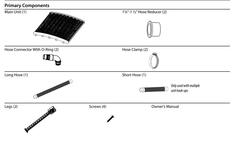
Note: Some parts may be pre-installed at the factory. Parts not shown to scale.
