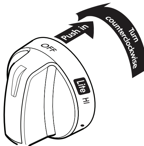
Figure 7: Proper way to turn on cooktop burners
