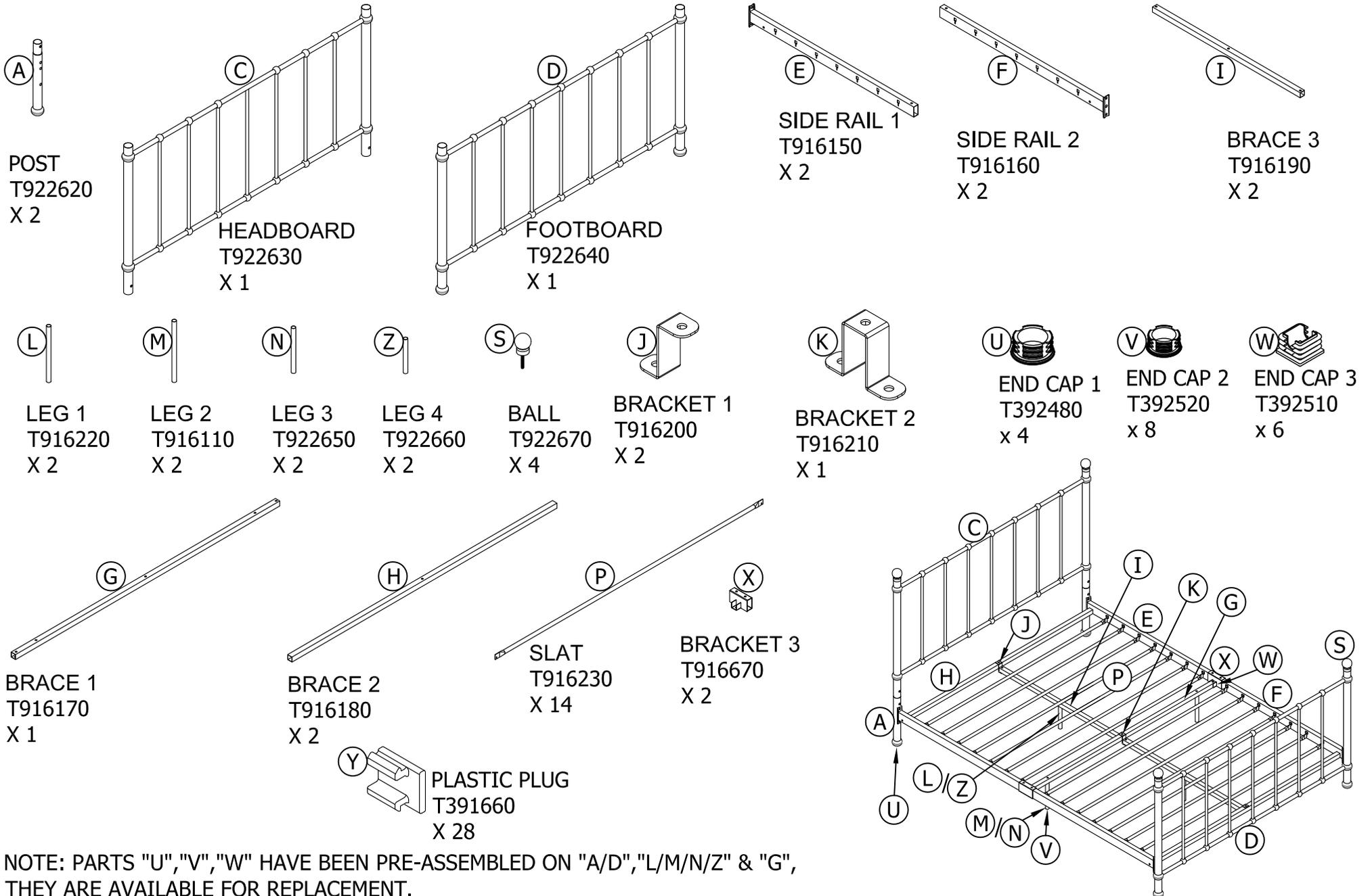
NOTE: PARTS "U","V","W" HAVE BEEN PRE-ASSEMBLED ON "A/D","L/M/N/Z" & "G",
