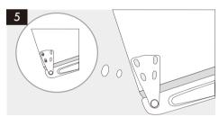
Insert top bracket hinge pin into hole in top of door. Use the two previously removed screws to attach back of top bracket to cabinet. Be sure to align the paper gasket beneath the two attachment holes in bracket.
