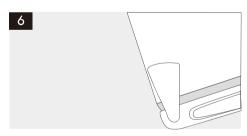
Replace the plastic hinge cover over the top hinge bracket.
