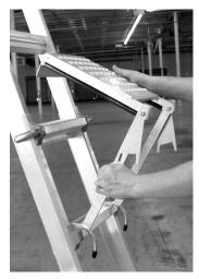
1. Place the wire hooks on the rung below the desired platform height. Place the Work Platform on the rung above the wire hooks. Ensure the Work Platform is securely in position before use.
