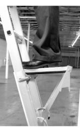
3. Push the Work Platform back with toe until the forward edge of the Work Platform rests securely against the rung. Ensure the Work Platform is securely in position before putting full weight on it.
