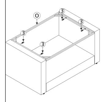
Connect the pasrt from STEP 9 & Table Top Frame (O) with Bolt (3)
