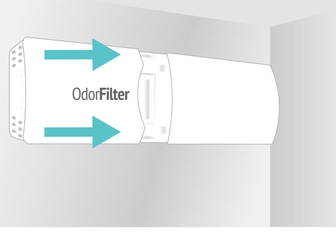
Step 5: Replace the cover of the compartment by sliding it back on
