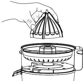
3. Remove the Reamer by grasping the Reamer and pulling up to remove it from the Drive Coupler.
