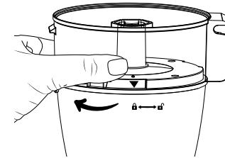
3. Turn Juice Bowl to your left until it locks into place and the Juice Bowl lines up with the lock graphic on the Motor Unit.
