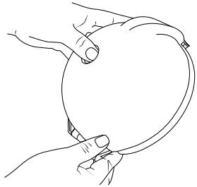
2. Remove the Holding Cone by tightly grasping the Lid with the domed part facing up. Firmly press down on the top of the Holding Cone to remove it from the Lid.
