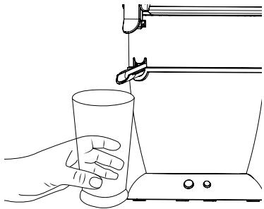
7. Place a glass under the Juice Spout. If the Juice Spout is in the UP position, the juice will collect in the Juice Bowl. If the Spout is in the DOWN position, the juice will flow freely into the glass.
