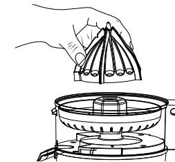
5. Place Reamer (D) onto Drive Coupler and Pulp Filter.
