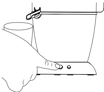
8. Press the Auto Juice Button. The motor will start, and the Reamer will automatically raise, extracting the juice. There will be a short pause; then, the Reamer will automatically lower. When the motor stops, the juicing is completed. The Auto Juice Button is illuminated solid blue during the juicing process, and reverts to flashing blue at the end of the juicing process.
