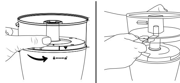
5. Remove the Juice Bowl (Ensure the Juice Spout is in the UP position). Grasp the Juice Bowl and turn counterclockwise until the arrow on the Juice Bowl lines up with the Unlock graphic on the Motor Unit. Lift the Juice Bowl straight up to remove it from the Motor Unit.
