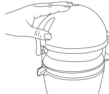
6. Close the Lid, ensuring the Lid is latched correctly so it will not open during the juicing process.
