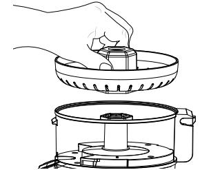
4. Position desired Pulp Filter (J or K) onto Drive Coupler.
