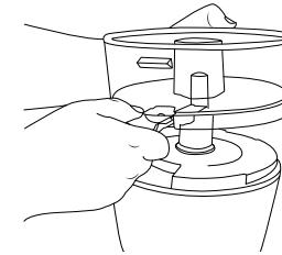
1. Place Juice Bowl (E) on to Motor Unit, lining up the Drive Coupler (M) on the Motor Unit with the hole in the Juice Bowl.
