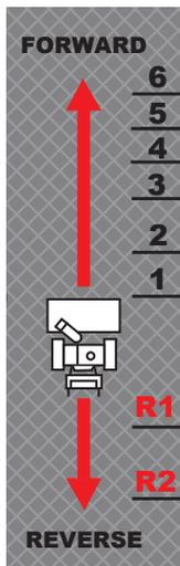
*There are six forward speeds and two reverse speeds. Release the drive control lever when changing speeds or direction.*
