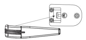
The base of the door handle is attached to the unit. Remove the pull handle that is packed inside the refrigerator.
