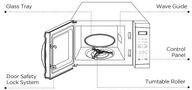
NOTE: Do not remove the mica plate covering the wave guide in the oven cavity.
