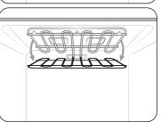
1. To change the bulb, you must tilt the broil heater down. To do this, turn the circular nut on the support counterclockwise while holding the broil heater. The broil heater should loosen and tilt down.
