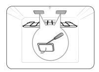
While holding the glass cover with one hand, insert a flat-sharp tool such as a table knife between the glass and the frame to remove the glass cover.
