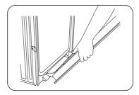
3. Hold the door at a 45° angle, and then align the door hinges with the slots in the lower front of the oven cavity. Slowly insert the door, making sure you maintain the 45° angle. You will know the door is engaged in the slot when you feel a slight drop.
